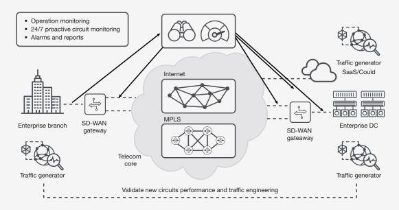
**Link verification** – Get real-time link analysis while running diagnostic tests on your network. Hawkeye enables you to do both at the same time.
